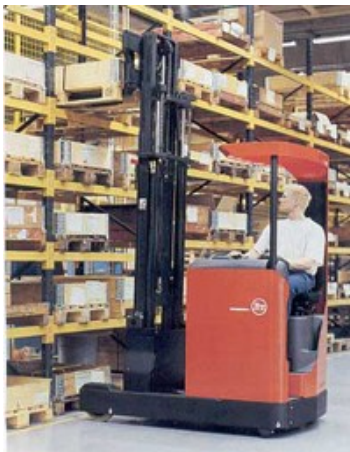
Figure 26 Reach Trucks / Fork Lifts
